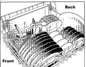
With the Stack–Rack shelf raised, thin items like cookie sheets or pizza pans may be placed along the left side. With the shelf down, two levels of glasses and cups can also be loaded.
